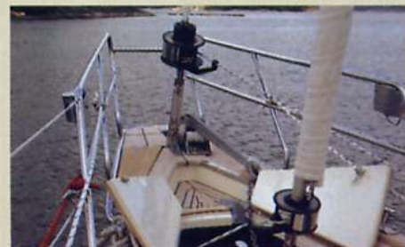
Top, the large chart table and abundant stowage round the navigating station. Above, the windlass is sited inside the anchor locker
